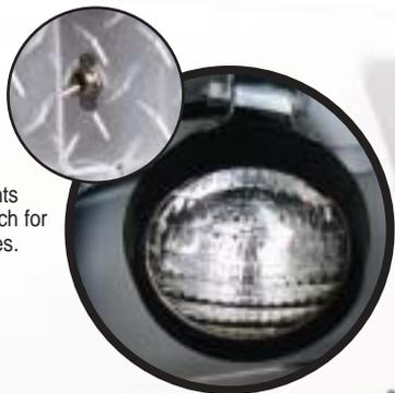
Two flood lights with rear switch for night deliveries.
