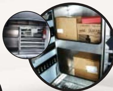
Bottle racks and shelving units bolted to front bulkhead leaving cargo area open.
