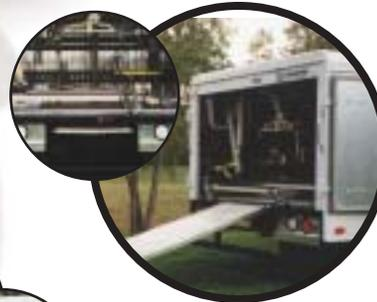
Aluminum bottle holders with access doors allow for easy access and storage of oxygen bottles. (E, M-6, D, G, H, Etc.).
