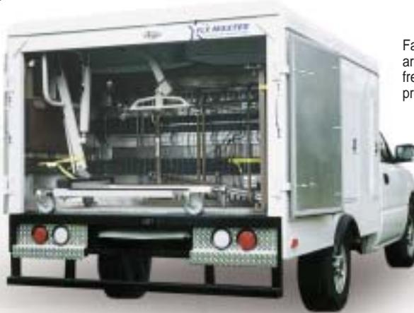
False ceiling provides storage area for mattresses. This frees up floor space and prevents damage.
