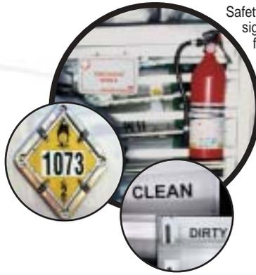
Brackets and slats mounted on interior side walls provide secure storage areas to avoid clutter and damage.
